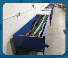
**Efficient Testing** Hoses are hydrostatically tested for 5 minutes to 1.5x the assembly's rated working pressure.
