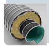
Thermo and insulating hose for maintaining cold or hot temperature air flows, asbestos-free insulation material, good sound proofing, flexible
