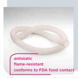
PU Suction & Transport Hose with stainless steel helix, **super lightweight**, antistatic,  $R_o < 10^9$ , flameresistant, hose wall conforms to FDA, **highly flexible**, smooth inside for optimum flow
