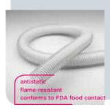
PU Suction & Transport Hose with stainless steel helix, medium/lightweight, antistatic,  $R_0 < 10^9$ , flameresistant, hose wall conforms to FDA, very flexible, smooth inside for optimum flow
