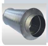
Sound attenuator, inner core perforated & corrugated aluminum, packed fiberglass insulation, outer core corrugated aluminum, mechanically fastened aluminum fittings on each end
