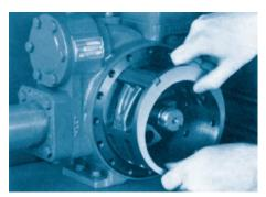
Easily replaceable liner restores efficiency.
