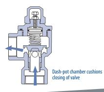
Blackmer differential bypass valves are designed to protect pumps and system components from excessive pressure damage, and no  $CO_2$  pump installation is complete without one. Blackmer offers five different models that provide full-flow pressure control to 250 U.S. gpm (946 L/min.) at 120 psid (8.27 bar). Installation is easy with NPT tapped ports in sizes from 3/4 in. to 2 in.
