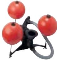
The unique FSP scum skimmer removes floating oils and grease solids. The scum is pumped from the skimmer to the concentration tank for processing.
