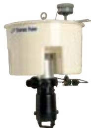
SBR and Digester decanting pump is equipped with a suspended solids sensor that allows the decanter pump to operate independently. When the suspended solids rise above the set value, the sensor will activate shutting down the decanter, ensuring that only supernatant water is discharged without any entrapment of sediment.
