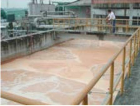
The BER is designed for both very high oxygen transfer and excellent mixing. The BER is used in Sequence Batch Reactors (SBR) where high oxygen transfer is required during the aeration cycle and excellent mixing only during the anodic cycle.
