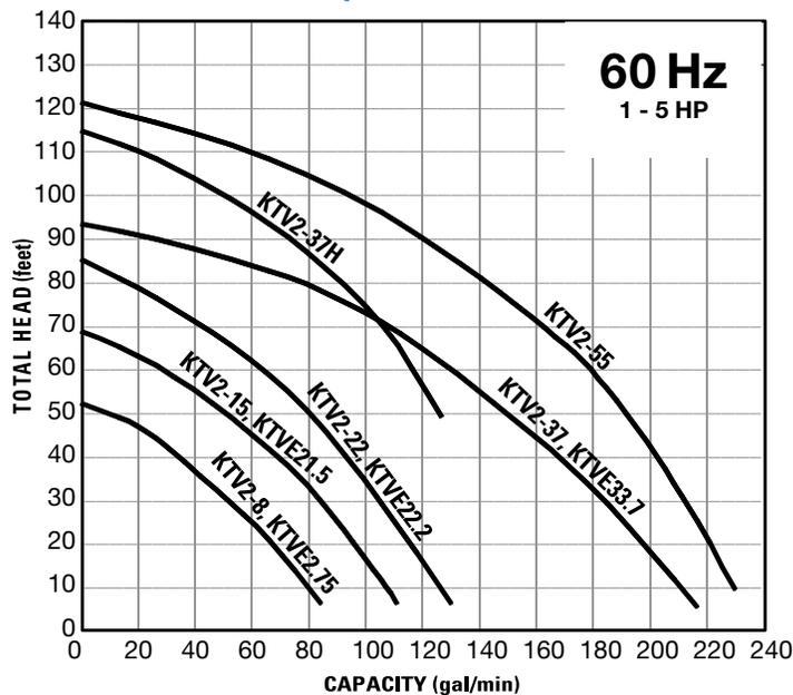
**KTV series** was developed with a die cast aluminum body and elastomer pump end to reduce weight and allow easy handling. The semi-vortex impeller allows for maximum particle passage size while offering increased parts life. In addition, the need for impeller efficiency adjustments has been completely eliminated.
