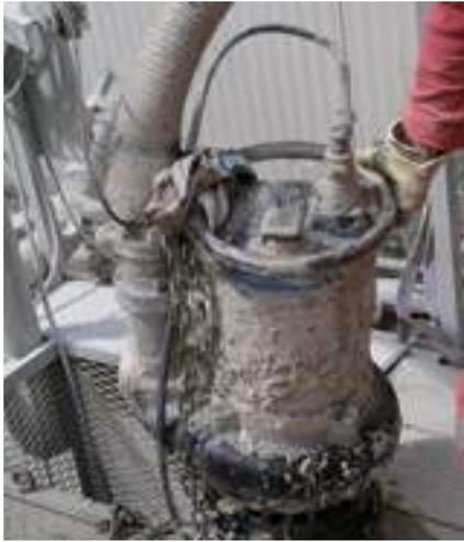
**Tsurumi Agitator Pumps** are designed for sludge slurry pumping with hard iron adjustable wear parts. Up to 10" discharge size / 100HP with 4 pole / 6 pole motors for slower impeller tip speed which prolongs pump life.
