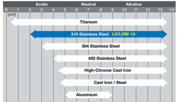
The above data is a rough indication for sulfuric acid (H<sub>2</sub>SO<sub>4</sub>) and sodium hydroxide (NaOH). Metals are affected by the type of acid/alkali, seal material, painting and abrasive environment.
