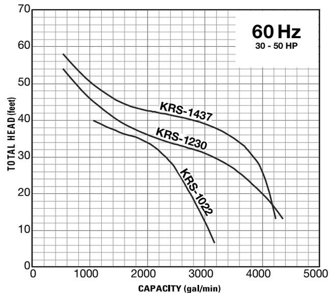
**KRS series** offers longer wear life on parts due to the slower impeller tip speed provided by 4-pole, 1800 RPM / 6-pole, 1200 RPM motors. Reducing impeller speed by half will extend your parts wear life by at least 2 to 3 times.
