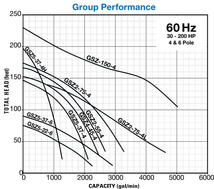
**GSZ series** is one of the most formidable high volume submersible dewatering pumps available. Reducing impeller speed by half will extend your parts wear life by at least 2-3 times. With impeller materials of High Chrome and Stainless Steel, the GSZ series tackles the most aggressive dewatering applications. The side discharge design allows a smooth passage of abrasive materials.
