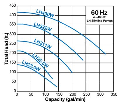
**LH Series** handles medium to high flows at higher heads, yet its top discharge flow-through design welcomes low water level operation for extended periods. Complete with a high chromium semi-open impeller and adjustable wear rings, our LH pumps provide you with increased wear resistance whether your application is construction site drainage, or commercial/ industrial mine dewatering, or effluent transfer.
