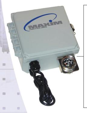
Each MAXIM controller comes ready to install with a stainless steel, mounted, differential pressure switch-gauge, enclosure mounting brackets and a standard 6 foot outdoor cord with a NEMA 5-15 120 VAC plug. The MAXIM includes a water-resistant electrical entry fitting and user-friendly quick-connect wiring points for simple installation without the need for tools. Each unit is factory tested and includes a detailed owner's manual.
