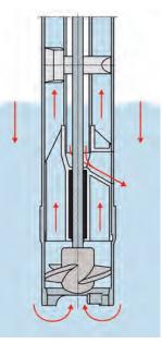
Optimal flow of the medium in the inner tube due to relief openings in the bearing housing.
