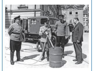
The world's first electric drum pump in operation.
