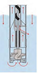
Optimal flow of the medium in the inner tube due to spiral shaped guide bearing.
