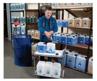
The pump FP 425 S in operation for conveying a particularly high-quality lubricant.
