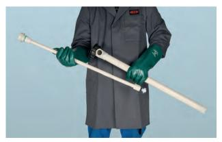
With just three hand movements the pump can be disassembled into inner tube (complete) and outer tube.
