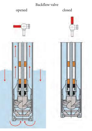
After pumping (left) the backflow valve is closed to remove the pump. The medium remains in the pump (right).
