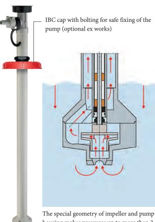
housing makes pressures up to more than 3 bar possible at high flow rates.
