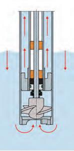
The mechanical seal prevents medium from getting into the inner tube while pumping.
