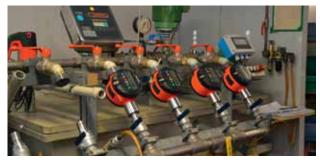
Each flow meter is checked and calibrated - 100 % quality control!
