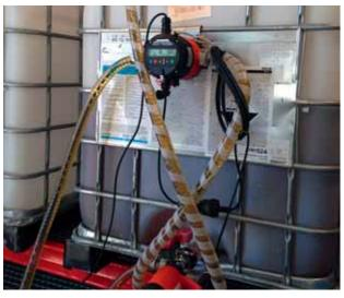
Semi-automatic filling with FMC 100 and switching amplifier FSV 100 from IBC.
