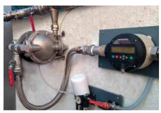
FMC 100 in combination with air-operated diaphragm pump for manual use.
