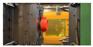
Own injection moulding production, here for the housing of an FMC.
