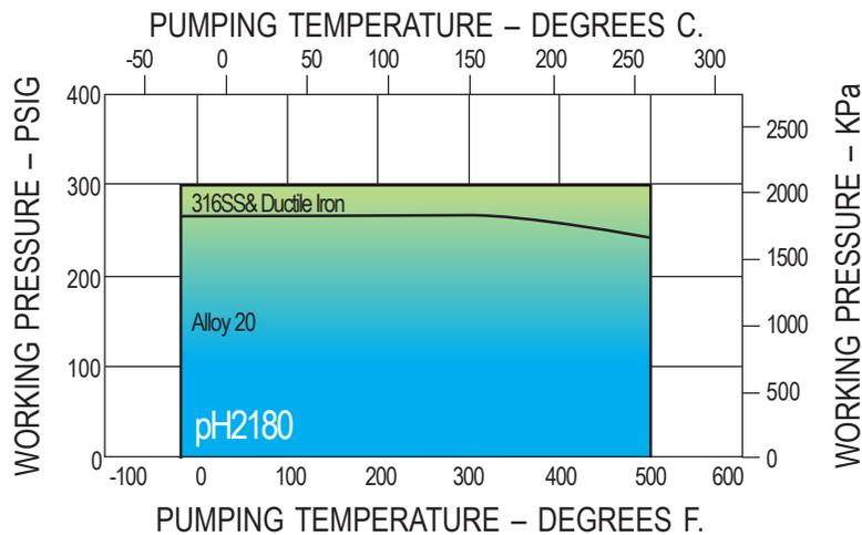
NOTE: For all Series pH pumps: lower temperature capabilities are available for special applications.
