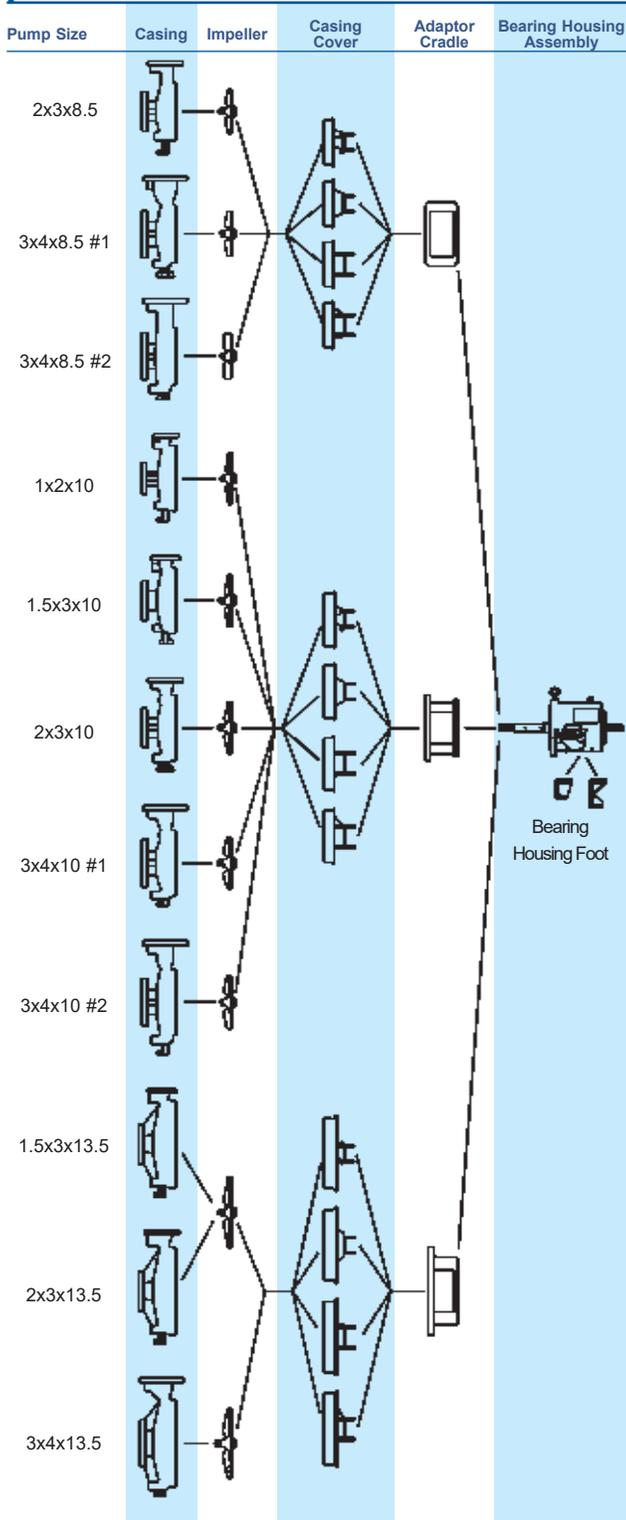
Casing covers with jackets, standard bore, large taper bore, and large cylindrical bore seal cavities are available on all pumps. Bearing housings with finned tube oil coolers are also available on all pumps.
