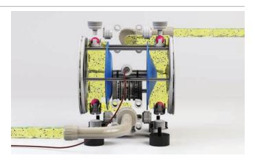
in the opposite direction. In the second figure, liquid is drawn in by the left-hand diaphragm and displaced by the right-hand diaphragm. The liquid is displaced – and thus conveyed – by the compressed air. The diaphragms merely serve as barriers and are not pressurized. This is a fact of decisive importance for the service life of the diaphragms.
