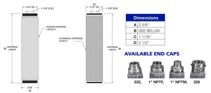
AMBF recommends not to flow more than 10 gpm per 10" cartridge at 40 microns and lower.
