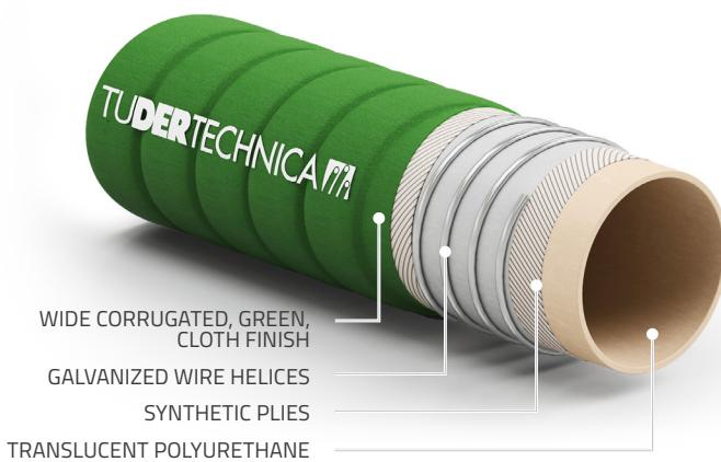
Suction and delivery hose suitable for powdery and granular dry food products.
