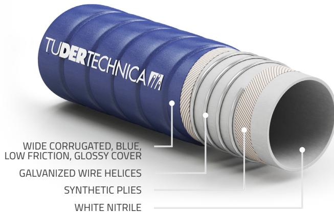
Extra flexible suction and delivery hose suitable for fatty and non-fatty food products. Hose tested according to the main norms for food contact materials (FCM – Reg. (CE) 1935/2004). Manufactured according to GMP (Reg. (CE) 2023/2006).
