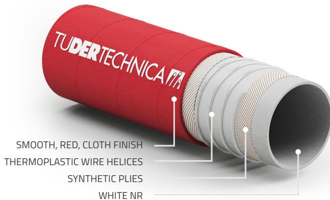
Suction and delivery hose suitable for milk, milk by-products, wine and non-fatty food products. Crush resistant. Manufactured according to GMP (Reg. (CE) 2023/2006).
