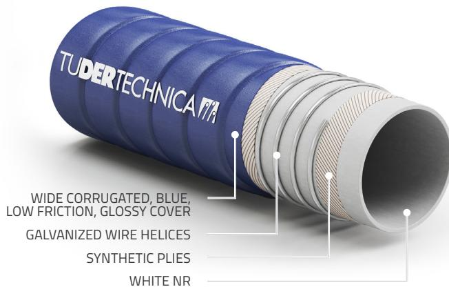
Extra flexible suction and delivery hose suitable for milk and milk by-products.
