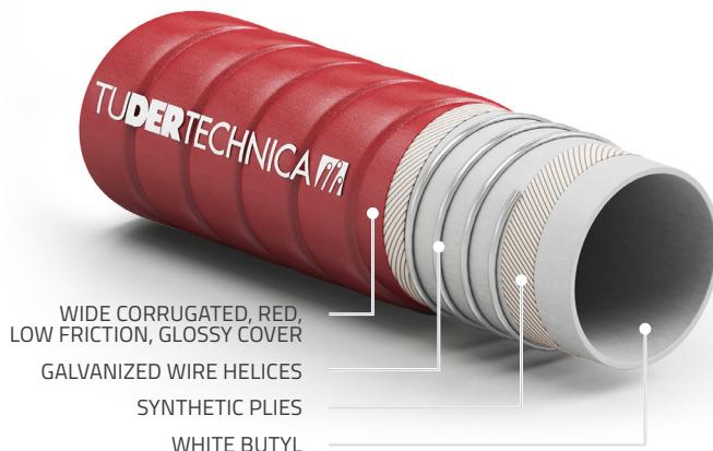
Premium grade low permeation extra flexible suction and delivery hose suitable for beer and a wide range of non-fatty food products with an improved resistance to higher pressure. Hose tested according to the main norms for food contact materials (FCM – Reg. (CE) 1935/2004). Manufactured according to GMP (Reg. (CE) 2023/2006).
