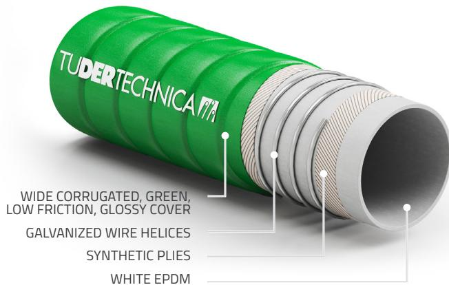
Extra flexible suction and delivery hose suitable for a wide range of food products. Not recommended for fatty food products and oil. Manufactured according to GMP (Reg. (CE) 2023/2006).
