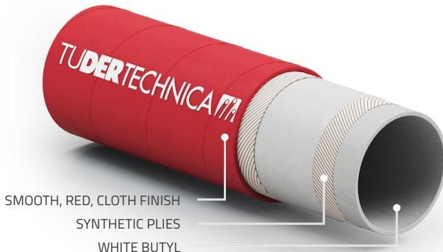
Premium grade low permeation delivery hose suitable for beer and a wide range of non-fatty food products with an improved resistance to higher pressure. Hose tested according to the main norms for food contact materials (FCM – Reg. (CE) 1935/2004). Manufactured according to GMP (Reg. (CE) 2023/2006).
