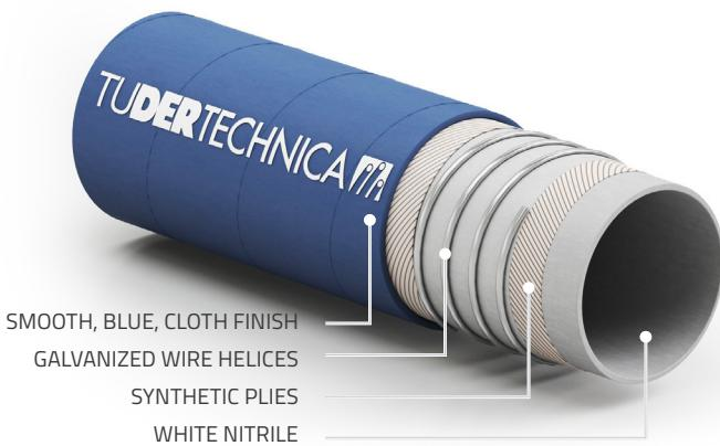
Light and flexible lorry collecting hose suitable for fatty and not fatty food products. Hose tested according to the main norms for food contact materials (FCM – Reg. (CE) 1935/2004). Manufactured according to GMP (Reg. (CE) 2023/2006).
