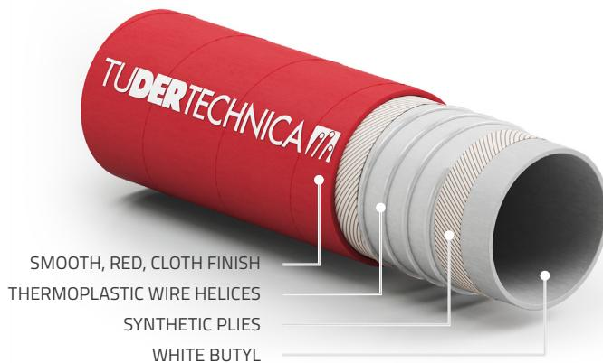
Premium grade low permeation suction and delivery hose suitable for a wide range of products. Recommended for wine and spirits. Crush resistant. Hose tested according to the main norms for food contact materials (FCM – Reg. (CE) 1935/2004). Manufactured according to GMP (Reg. (CE) 2023/2006).
