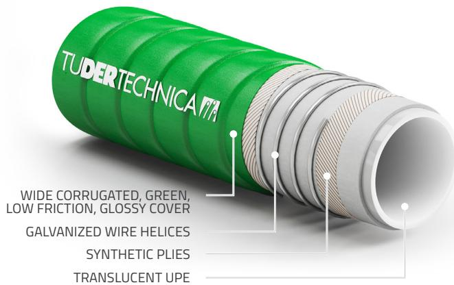
Extra flexible suction and delivery hose suitable for distilled and distillation by-products with alcohol concentration up to 99%. Hose tested according to the main norms for food contact materials (FCM – Reg. (CE) 1935/2004). Manufactured according to GMP (Reg. (CE) 2023/2006).
