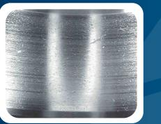
Abrasive or Hard Contaminants: Examples include dust, dirt, small metallic parts from machine wear or piping breakdown. These contaminants can begin to break down oil cleanliness and cause equipment problems in the hydraulic circuitry.
