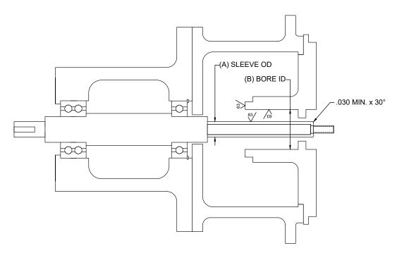
Figure 1: Surface finish and chamfer locations. Fully assembled pump without seal.
