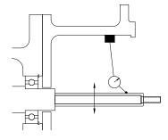
Figure 3: Bearing Fit
