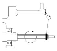
Figure 4: Bearing Frame Perpendicularity
