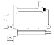
Figure 5: Axial Shaft Movement
