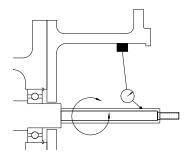
Figure 2: Shaft Runout
