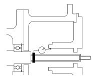
Figure 6: Seal Chamber Bore Concentricity
